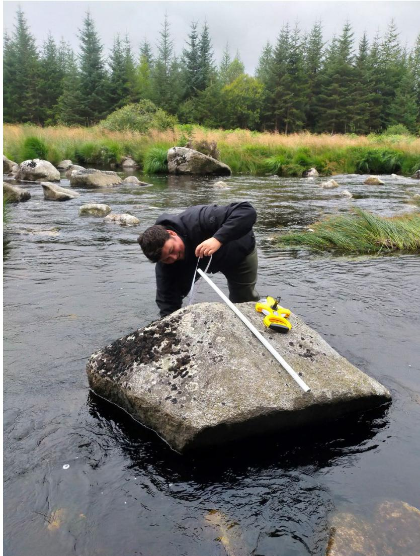
*Figure 2: Measuring the distance between the top of a solid structure to the river bed using a flat stick and measuring tape*
