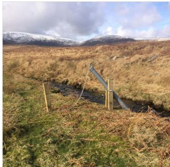
*Figure 2: GFT's framework which is used to house and protect the sondes whilst deployed in the field*
