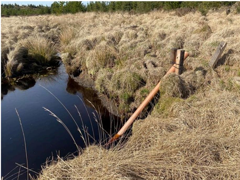
*Figure 30: Site 1 sonde placement in a corner pool on the Dargool burn. Picture taken at low water on the 22/04/2020*
